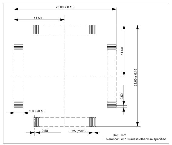
Figure 6 Recommended Dimensions for Mount Pad
